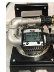
Fig. 4. Sampling device with filtered volume and flow rate visible.
