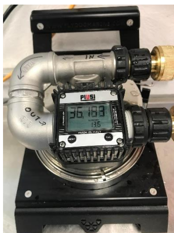
Fig. 4. FerryBox sampling device with filtered volume and flow rate visible.
