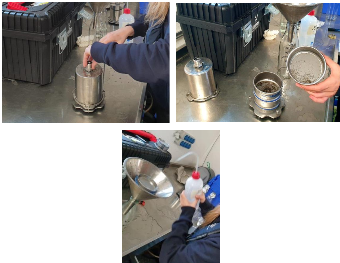
Fig. 3. Disassembling the FerryBox sampling device and sample collection.
