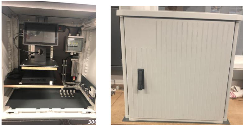
Fig. 8. Cabin with NVR included. On the left the interior of the cabin is shown. The image on the right represents the exterior of such a cabin.
