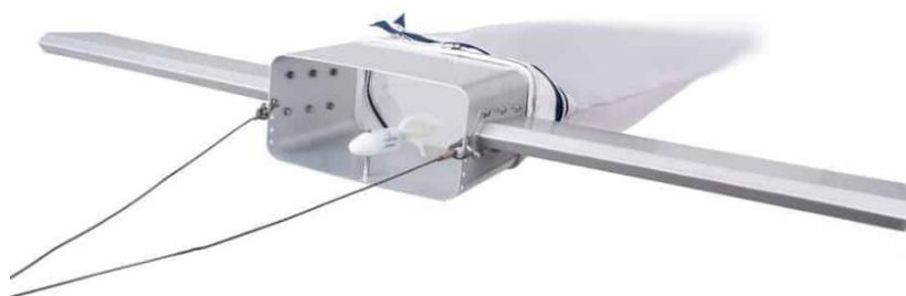
Fig. 1. Example of manta net model to be used in the sampling activities of INSPIRE (source: Hydro-Bios).
