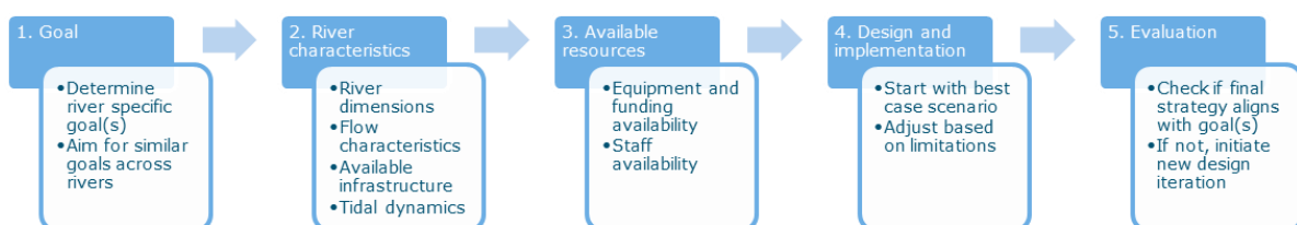
Fig. 13. Workflow for developing a targeted river plastic monitoring strategy following a harmonized approach [adapted from van Emmerik et al. (2023)].
