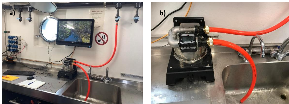
Fig. 2. a) General overview of the FerryBox device, connected to a pumping system available in a research vessel; b) Detailed image of the assembled collection module, with a connection for water input and output. Photo credit: Nelle Meyers, ANDROMEDA JPI Project ( www.andromedaproject.net ).
