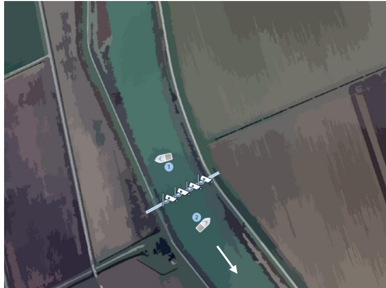
Fig. 4. Schematic of release-catch experiments for validation of bridge-mounted camaras. Legend: 1 and 2 – Locations A and B for the release/catch points depending on the tide.
