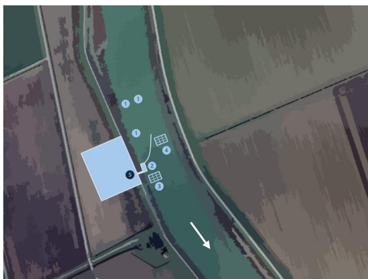
Fig. 9. Schematics of release-catch experiments for technologies at freshwater abstraction points. Legend: 1 – potential locations for the release point, 2 – collection from the technology and around it, 3 – collection after the technology, 4 – collection of plastic litter not intercepted, 5 – collection of plastic litter in the treated water.
