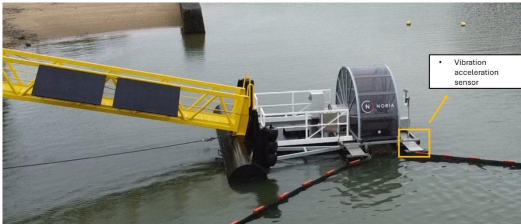
Figure 35: INSPIRE's vibration acceleration sensor mounting location on CirCleaner.
