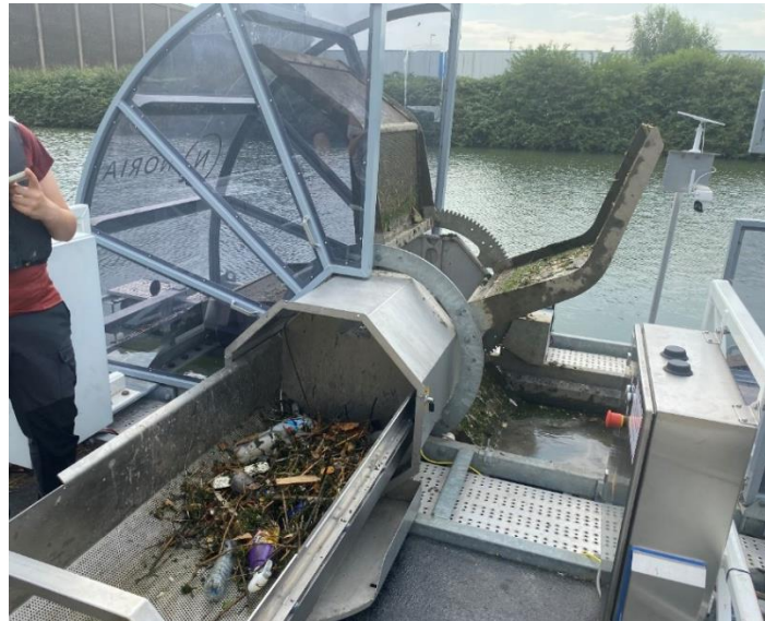
Figure 32: CirCleaner's collection compartment (Photograph by Jan Puhar).
