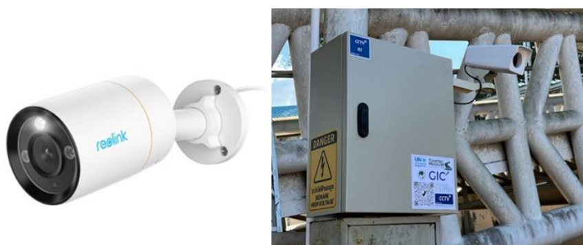
Figure 9: Camera systems used within INSPIRE: RGB RLC-1212a 4 mm camera (left) and pLitterCCTV unit with housing mounted on a bridge (right).
