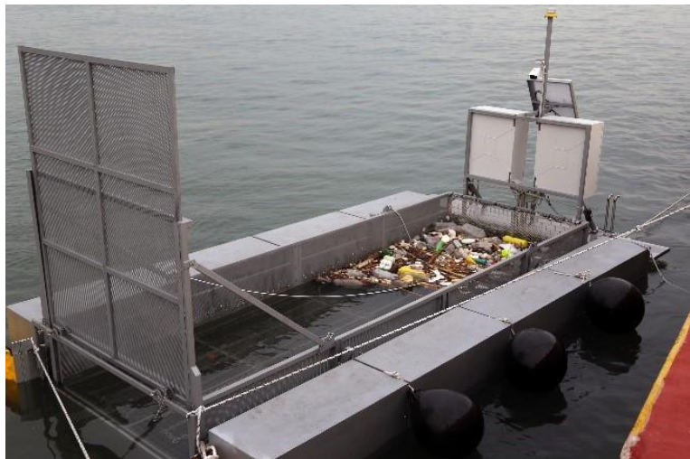
Figure 21: CLEAN TRASH collection cage, developed in CLAIM project.
